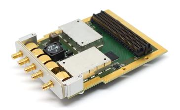
The Creonic L-band RF receiver FMC card allows receiving RF signals between 925 and 2,250 MHz. It is ideally suited for satellite communication with standard satellite dishes since it includes a DiSEqC driver IC for LNB controlling. Due to the low-pin-count (LPC) FMC connector it can be used with all FMC carrier boards that support  $V_{adj} = 1.8V$ .
